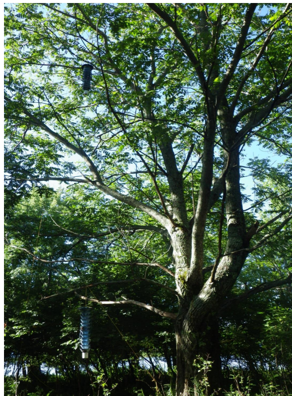
Figure 1. A 12-unit Multiple-funnel trap installed in a mature green ash ( Fraxinus pennsylvanica Marshall) at (a) the conventional height of chest level and (b) in the upper crown of the tree.
